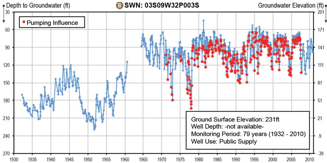
**B** Hydrograph 03S09W32P003S: Shows the successful recovery of groundwater levels associated with use of recycled and imported water in lieu of pumping groundwater, and conjunctive management of surface water and groundwater supplies.
